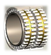
These bearings are designed for extremely high radial load capacity with case-carburized steel materials for race and rollers maximize resistance to shock, wear and debris.
